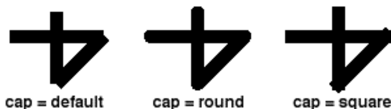
Figure 29: Example of lineMode attribute "cap"
